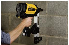
If you have larger numbers of fixings to make in one go, particularly straight onto brickwork, blockwork or concrete, then gas nailing is the way to go. In our trials, we used the <code>DeWalt® C5 gas nailer</code> with <code>25mm XC nails</code>. Once set up, the gun will fix nails straight through the pre-formed hole or even
